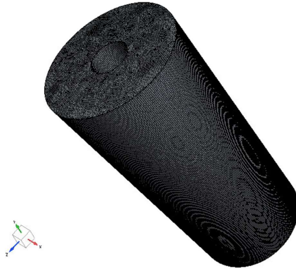
Figure 29: The finalized CC27 mesh with a base size of 0.30 mm and cell count of 2,313,608 cells. The outside and upper surface of the cup geometry is visible.
