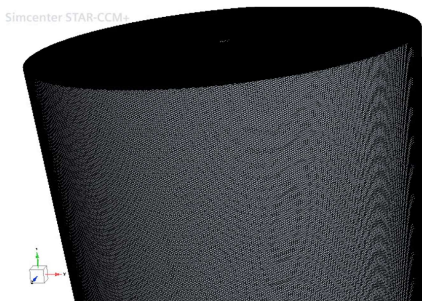
Figure 63: RV5 0.40mm base size final production mesh.
