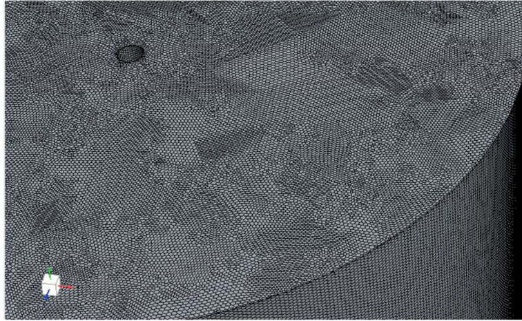
Figure 30: The finalized RV5 mesh with a base size of 0.40 mm and cell count of 3,783,388 cells. The outside and upper surface of the cup geometry is visible. Figure is zoomed in to visualize the contour of the cells, another Figure is available in Appendix C1.
