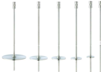
Figure 7: RV spindle-set for the Brookfield viscometer, RV2-7 in order left to right. (AMATEK Brookfield, 2026)
