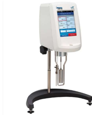
Figure 6: Brookfield DV2T-RV Viscometer. (AMATEK Brookfield, n.d.)
