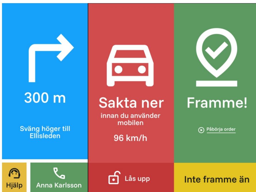
Figure 4.6. Static mid-visual fidelity prototype of GPS-based context-aware views and constraints, including turn-by-turn navigation guidance, a velocity-based interaction lock, and an arrival state with a start-order action.
