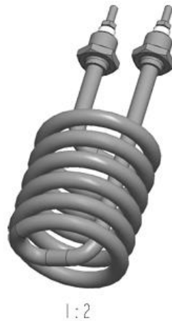
Figure 9: Example of a detail for which the scale differs from the main scale
