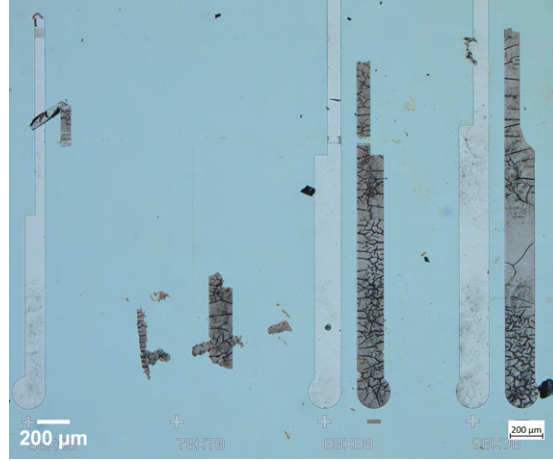
Figure 6: (a) Micrograph of silicon chip after the fifth experiment. This sample first was coated with the sugar solution and then placed in the oven at room temperature. The oven was shut-off, applying no higher temperature.
