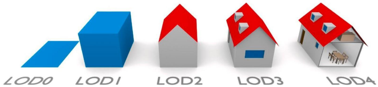
Figure 2.7: Representation of the LOD of CityGML 2.0 (Biljecki et al. 2016, p. 26)
