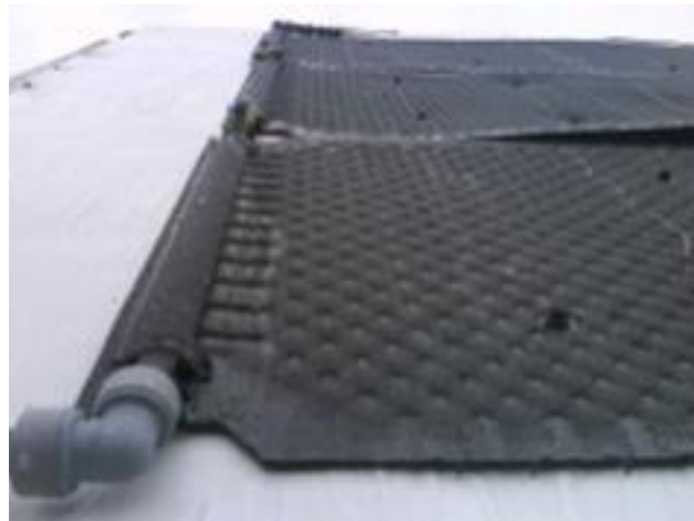
Fig. 1.2: Typical example of a WISC, designed to abstract thermal energy from a PV panel. Source: Mehnert et al., 2017.
