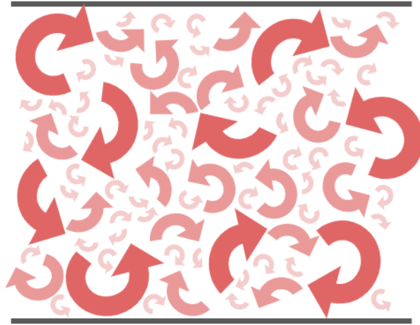
Figure 6: Cascading effect, where large eddies turn into smaller eddies.
