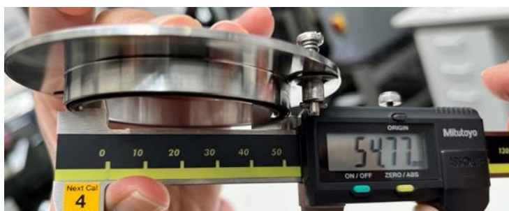
Figure 7. Measurement of the circular sample holder used to define coating area. The diameter of the test region is 54.8 mm, as measured using a digital caliper
