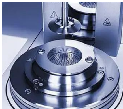
Figure 2. Anton Paar Immobilization cell showing perforated lower plate for suction-assisted dewatering and the upper geometry.
