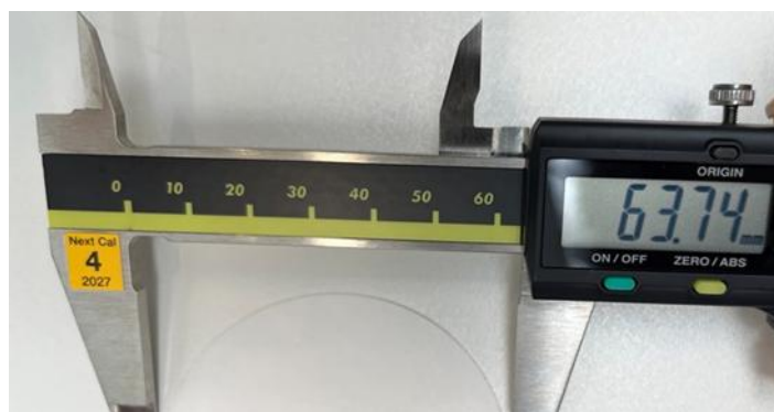
Figure 5. Diameter of circular paper substrate used in IMC experiments
