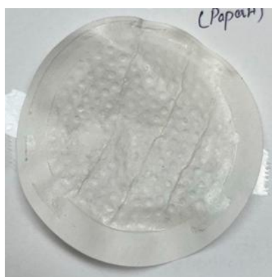
Figure C 1. Coated PVOH sample on paper A
