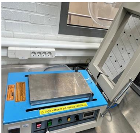
Figure 10. Film applicator (Rod coater), used for film coating
