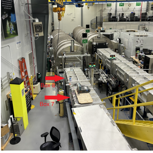
Figure 1: GP-SANS beamline at HFIR. The red arrows indicate the positions of boxes 7 and 8. A cylindrical neutron detector is located downstream of these boxes. Image by Linus Persson.
