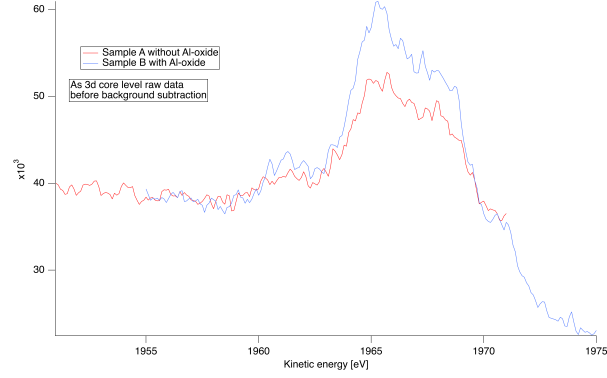
Figure 20: The range of the same core levels was different for both samples, such that the energy range used in sample A (red curve) cuts off a contribution as suggested by the spectrum from sample B and the clear shoulder at around E_k \approx 1970 eV.
