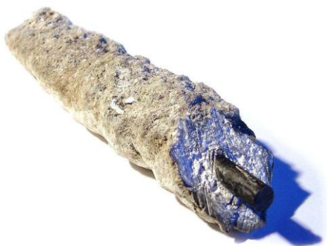
Figure 12. Biorock grown in the Maldives on a steel bar with 6 mm in diameter for around one year, reproduced from Goreau (2012), CC BY 3.0
