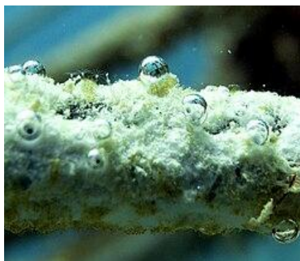
Figure 11. Bubbles from the hydrogen gas emerging from the growing material (the white layer), reproduced from Marionpinta (2011), CC BY-SA 3.0
