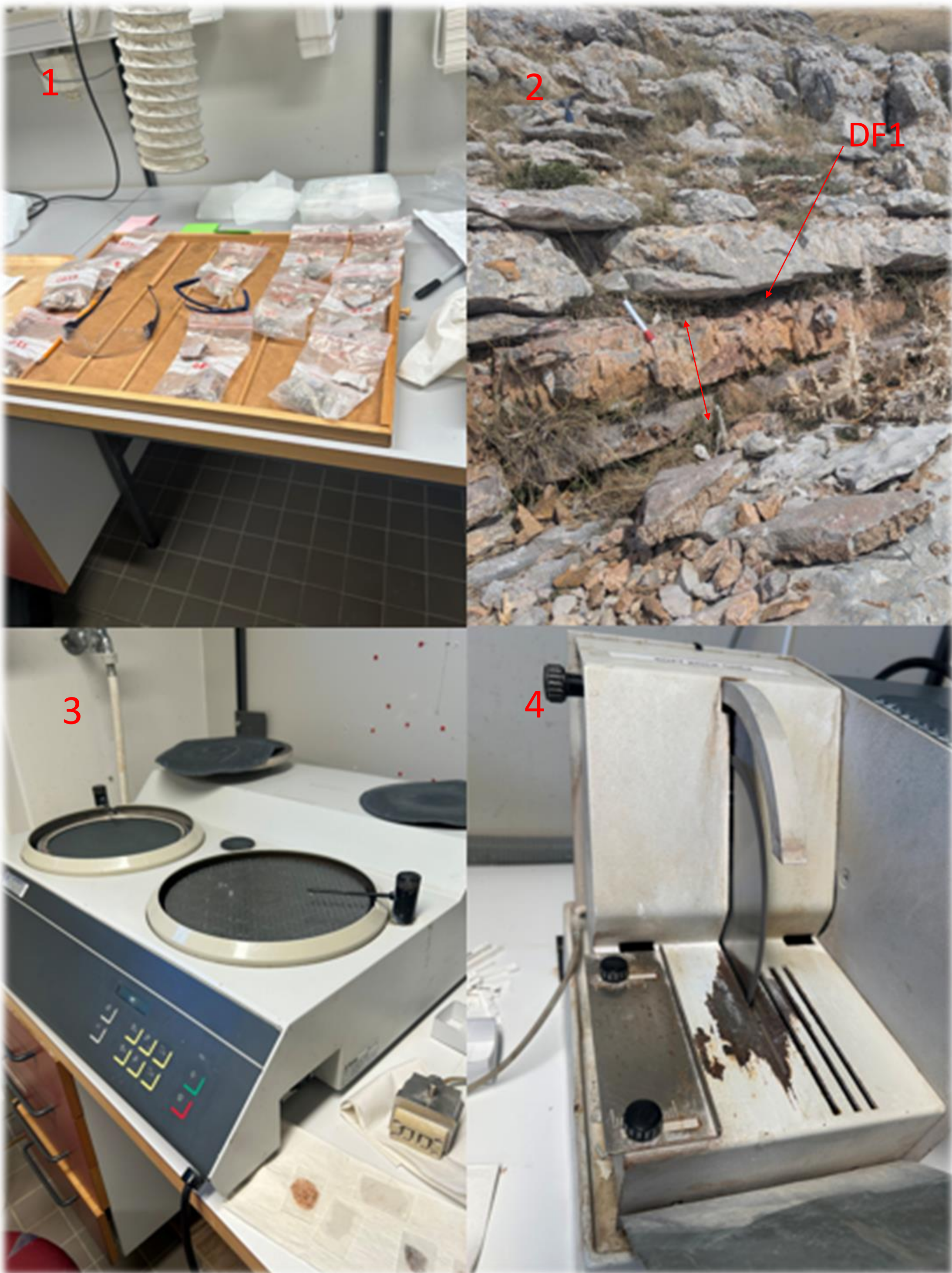
Figure showing method processes for this study. 1: All eleven samples in plastic bags in the thin-section laboratory. 2: density flow 1 (DF1) in field. 3: The sandpapering machine. 4: The sawing machine.
