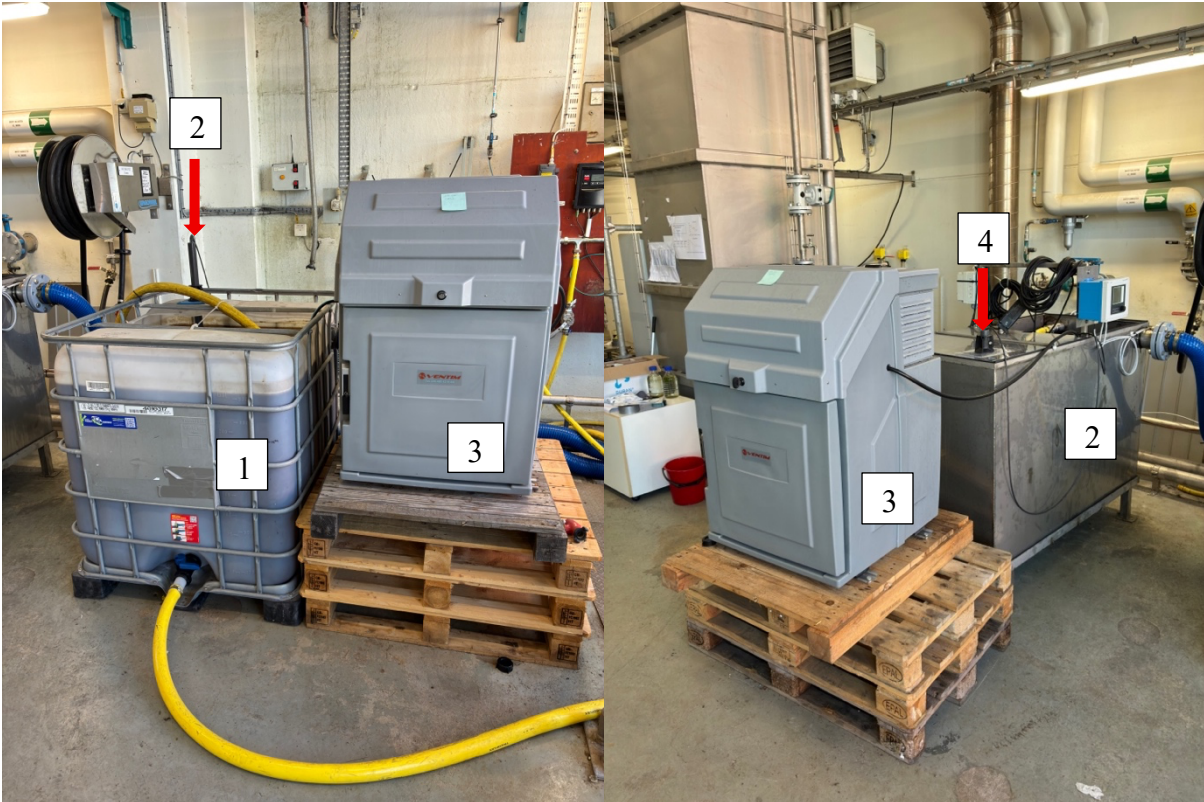
Figure 3.4. The numbers correspond to: 1 (influent tank), 2 (effluent tank), 3 (autosamplers), 4 (turbidity sensors).
