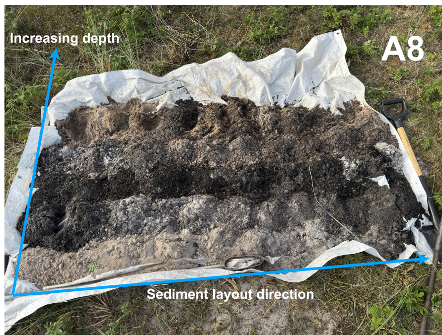
Fig. 11. Disturbed sediment samples recovered from auger hole A8 and laid out on a tarpaulin in stratigraphic order for field description and photographic documentation. Photograph by Shengliang Dong, 30 September 2025.
