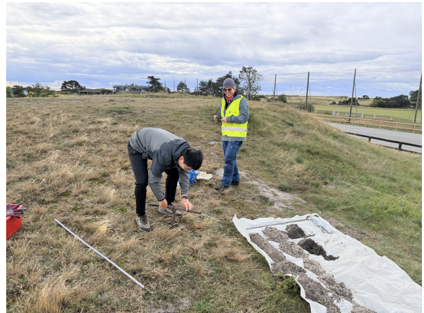
Fig. 9. Hand Auger sampling at Kolabacken. Photograph by Dan Hammarlund, 29 September 2025.
