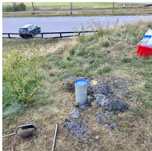
Fig. 41. Borehole B4 and the hand auger equipment used. Grey sand and coal fragments dug from the surface layer are visible around the borehole. To prevent collapse of the poorly consolidated sediments of Unit 1, a steel pipe was lowered into the borehole during augering. Photograph by Shengliang Dong, 29 September 2025.
