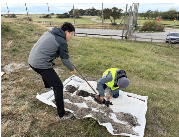
Fig. 12. Collection of POSL sample from the hand auger. Photograph by Dan Hammarlund at Kolabacken, 29 September 2025.
