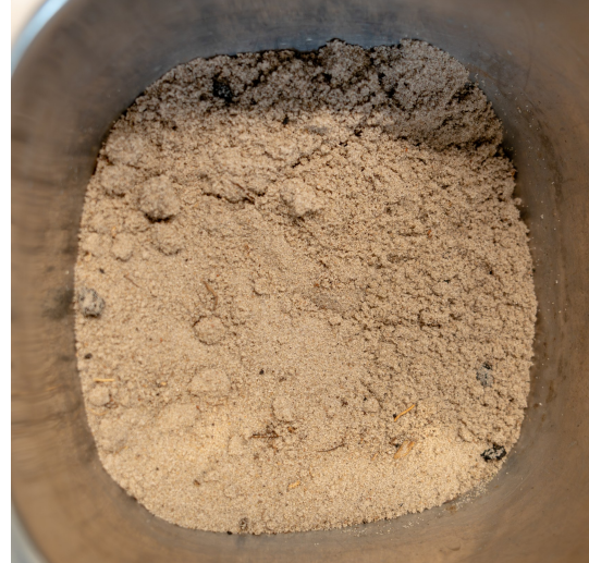
Fig. 32. Material from Unit 6: Whitish grey sand. Sample position: A10, 30 cm.
