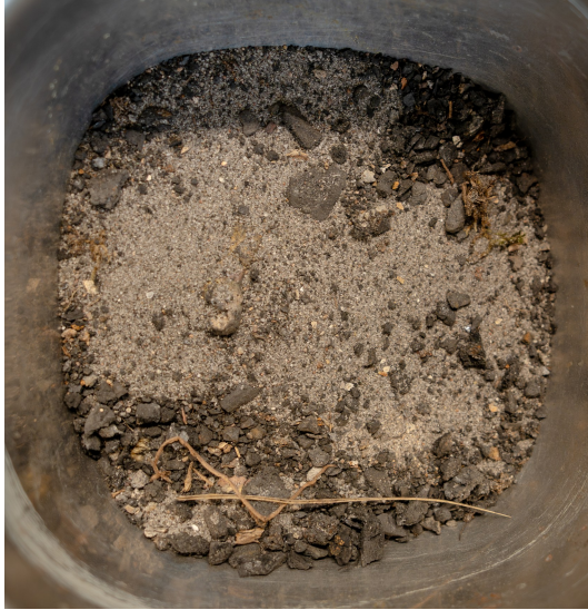
Fig. 30. Material from Unit 5: Grey sand with burnt coal. Sample position: A8, 112 cm.
