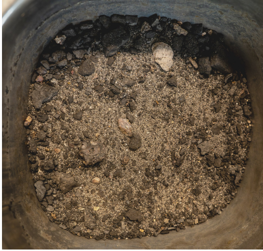
Fig. 26. Material from Unit 3: Black sand with coal particles. Sample position: A5, 201 cm.
