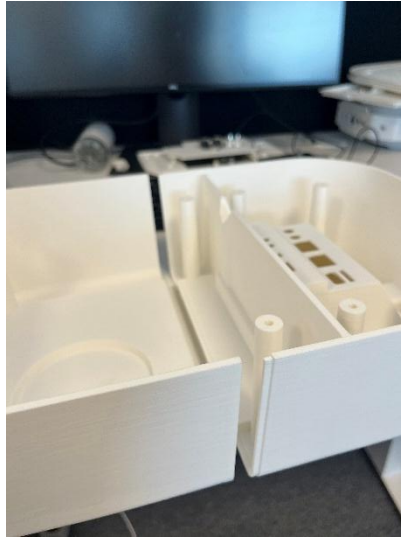
Figure 38 Split body operation results in 3D-printed model
