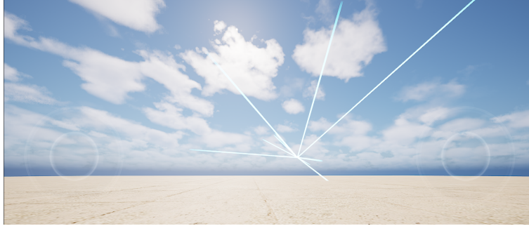
Figure 3.2: First in-engine visualization of the synthetic rays using Unreal Engine’s Niagara particle system. The light blue beams represent the MPCs.
