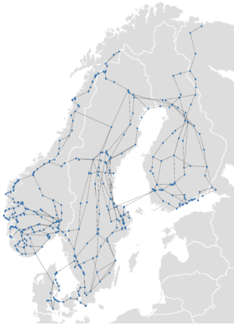
Figure 3.3: This figure was produced by extracting and processing data from the PyPSA network. It shows the spatial placement of the Nordic power grid nodes according to their geographic coordinates, overlaid on a public domain Nordic map [41].
