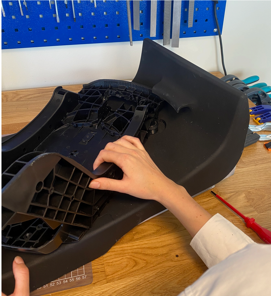
Figure 39 Milled seat frame installed on the prototype.
