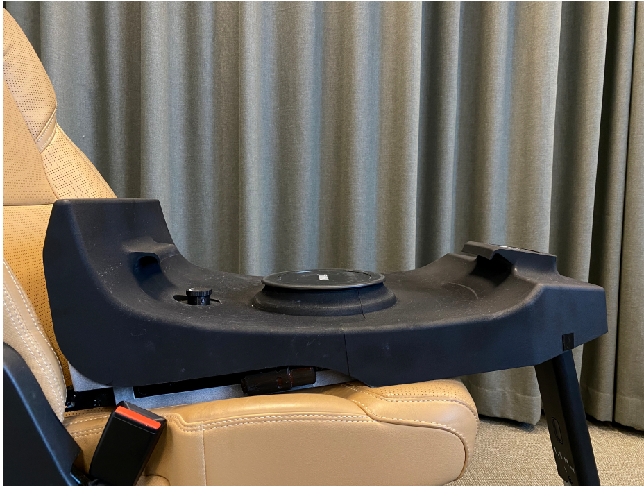
Figure 35 Lowest inclination of the base.
