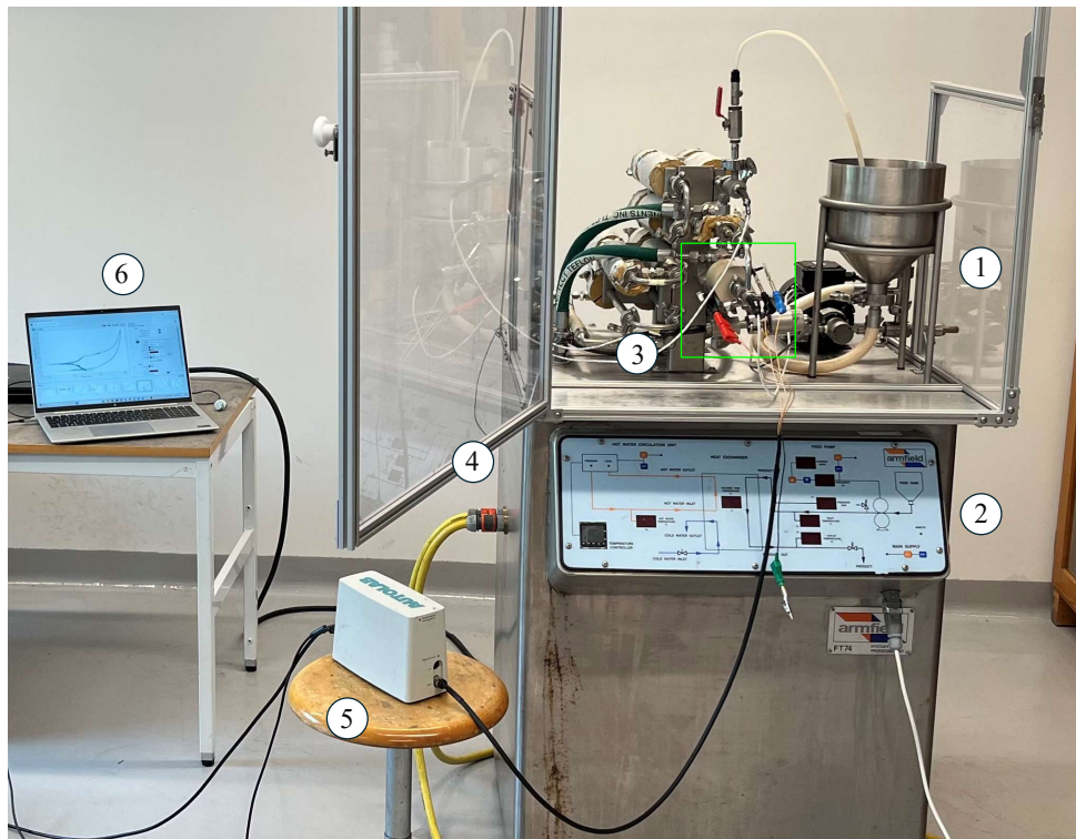
Figure 7: Test processing unit (Sören) and setup: (1) Pasteurizer. (2) Temperature and flow are controlled in the panel. (3) Test chamber. (4) Supply of cold water. (5) Potentiostat. (6) Software at computer to control and measure CPDP.
