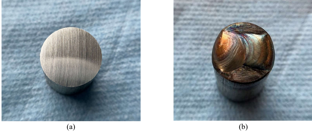
Figure 9: (a) Example of base SS grinded sample without welding. (b) Example of a 254 SMO SS sample after welding, without any grinding treatment applied.
