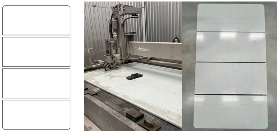
Figure 6.4 Cutting out the honeycomb plates
