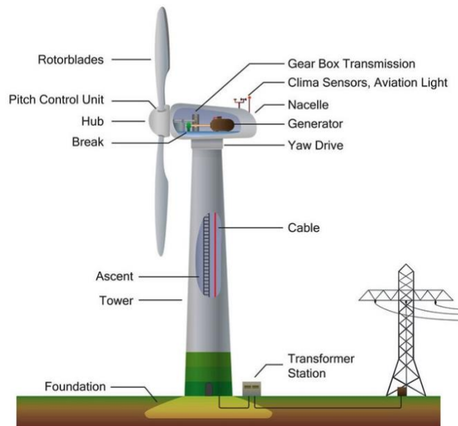
Figure 3. Main components of wind turbine (Bilderzweg – stock.adobe-com, 2022)
