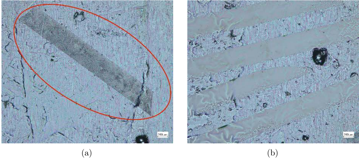
Figure 10: Optical micrographs of Alumel (K − ) poles from the latest batch thin sugar layer, corresponding to the geometry observed prior to liftoff in Figure 6(b), following transfer onto a polished stainless steel receiver substrate via reflow at \sim 70^\circ\text{C} and dissolution of the sugar carrier in water. Scale bars: 200\,\mu\text{m} .
