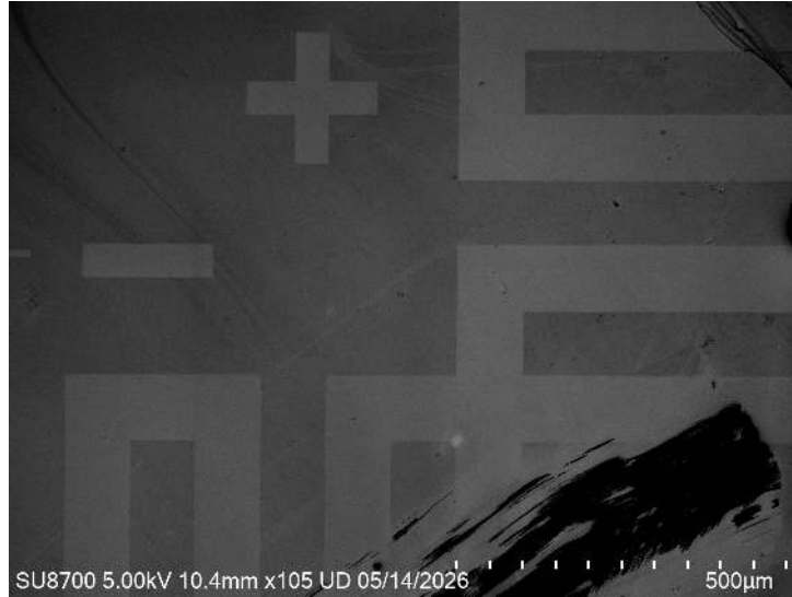
Figure 12: SEM image of the junction region where the Chromel (K+) and Alumel (K-) poles overlap on the latest batch sample variant B donor chip following attempted liftoff, imaged using the UD detector. Scale bar: 500 \mu\text{m} .
