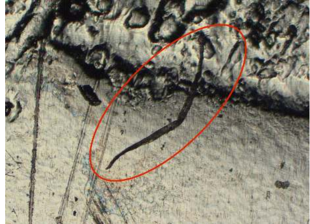
(b) Transferred Almel (K-) pole on stainless steel substrate.
