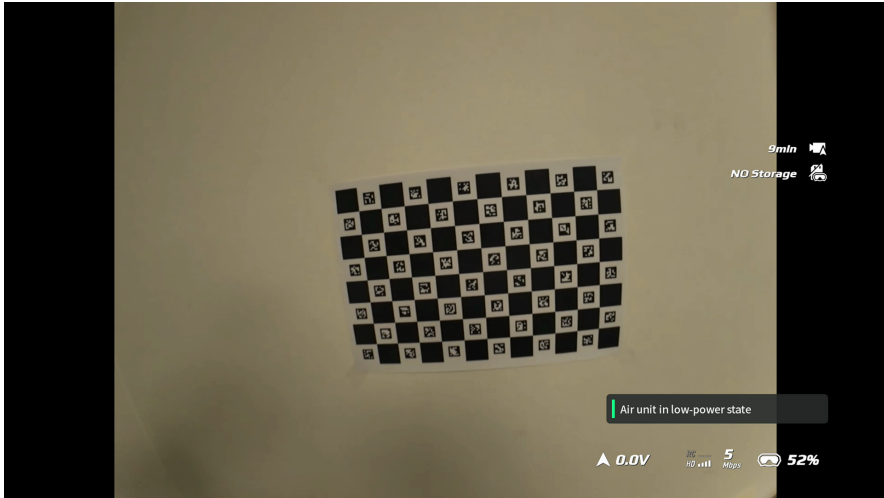
Figure 3.7 Example of a Charuco board used for camera calibration.
