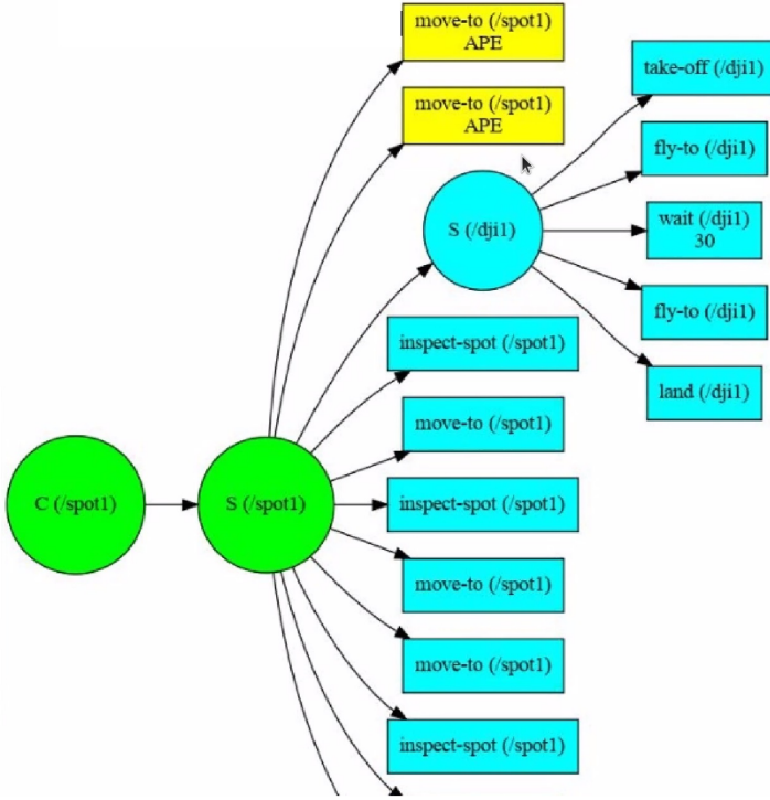
Figure 7.2 A fragment of the Task Specification Tree (TST) converted from the plan solution using TST factory in the WARA-PS framework: The corresponding TST uses elementary action nodes, corresponding to elementary actions of type inspect-spot , move-to , fly-to , etc. Furthermore, it requires a concurrent node (marked C) specifying that the actions can be performed concurrently, as well as a sequential node (marked S).
