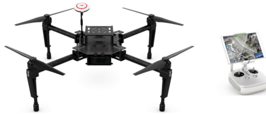
Figure 9.4 A DJI Matrice 100 (UAV) quadrotor with iPad. The DJI Matrice 100 platform is aimed at researchers and developers and is characterized by good access to the flight functionalities using the provided SDK. Its open construction provides possibilities of easy integration of additional components such as sensors or computational power. Courtesy: [WARA-PS, 2024]
