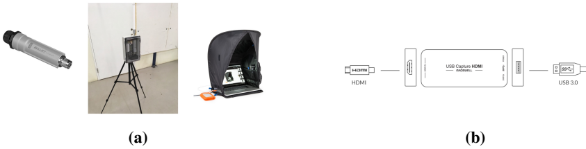
Figure 9.6 (a) DJIM100 Ground Station Equipment. Left: Bullet Titanium M5HP Access point. Middle: Ubiquiti complete base station to provide WiFi connectivity. Right: Laptop with screen sun protection. (b) Universal HDMI frame grabber which interfaces with the host PC using USB3.0 interface. (courtesy: [WARA-PS, 2024])
