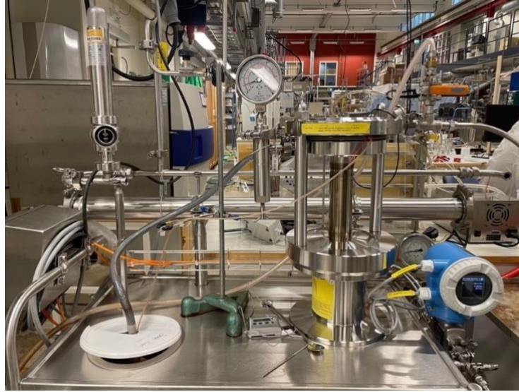
Figure 3.1. Experimental membrane filtration setup (Alfa Laval TestUnit M20).
