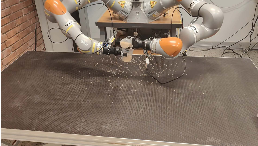
Figure 5.8: Representative snapshot of the Multi-view Baseline Policy spillage failure: rice is spilled outside the target container during the pouring process due to unregulated end-effector motion.
