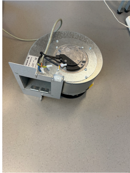
(b) Comsys cooling fan.
