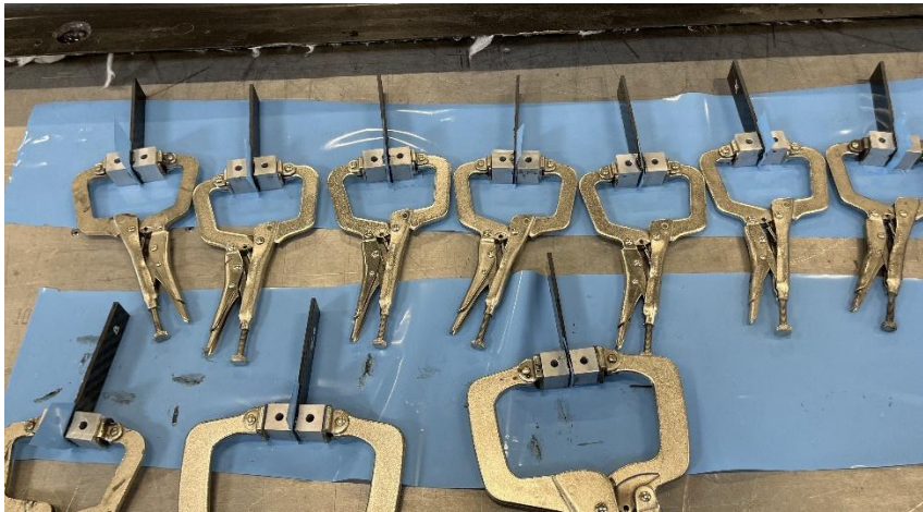
Figure 10 - Clamping of MDCB assembly post application of adhesive
