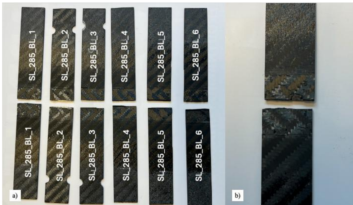
Figure 15 – Fracture surfaces for a) - SL_285_BL group. And b) -Up close fracture surface for one SL_285_A sample.
