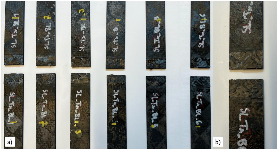
Figure 23- Fracture surfaces for a) - SL_Tx_BL_group. And b) -Up close fracture surface for one SL_Tx_BL sample.
