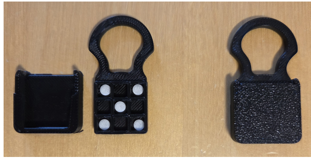
Figure 29: To the left, positioning of five pellets in an open 3D-printed holder with capacity up to nine pellets. To the right, an example of what the 3D printed holder looks like when closed.
