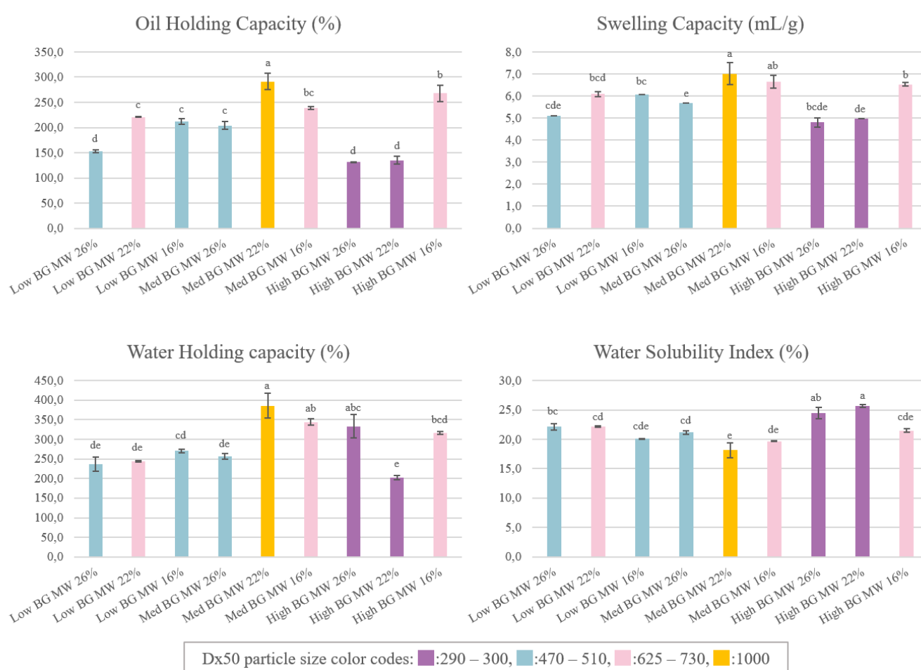
Figure 4.11. Oil holding capacity, swelling capacity, water holding capacity and water solubility index for ODBP samples that have been dried from different TS levels and with different BG Mw. All bars except one represent duplicate measurements. The swelling capacity for ODBP with high BG Mw and 22 % TS was measured once. The letters indicate statistical significance according to the Tukey test.
